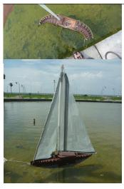
2010 08 16 : v002 Protei002 is the same size as 001, same remote control and electronic system on board. 002 is articulated, the entire body acts as steering : powerful, precise, rugged.
