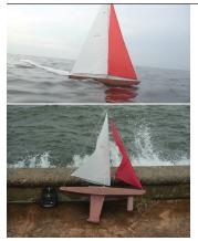
2010 06 22 : v000 Built in a day with plastic bags and duct tape, we tested this 1m inflatable prototype. It sailed in a gentle breeze with an articulated front steering.
