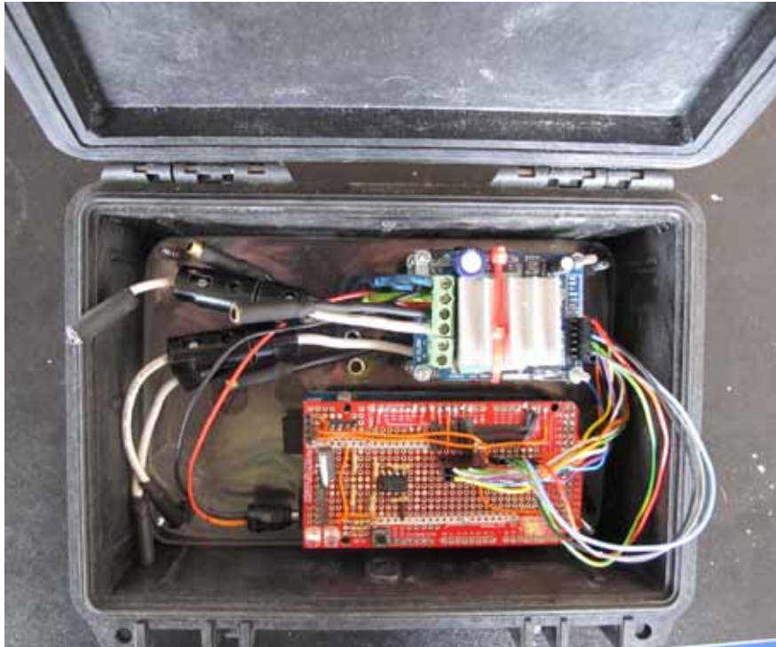
Figure [x]: The mounting of the Arduino Mega (with shield), and the two motor drivers (stacked on top of each other) inside the waterproof Pelicase. The colorful cables on the right connect the shield to the motor drivers, and the thick wires on the left provide connections for the motor cables (which enter through a tube on the back of the Pelicase).
