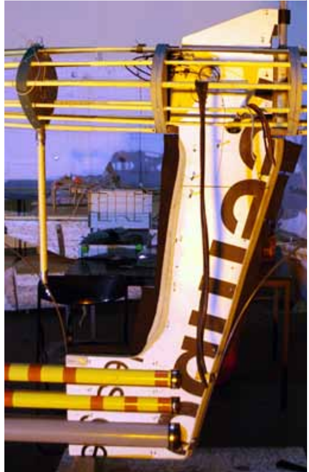
Fig. Finished keel with linear actuators, batteries and ballast mounted
