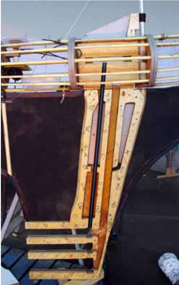
Fig. Inner structure of the keel
