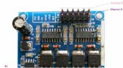
Figure [x]: The motor driver board used for driving the actuators on Protei.
