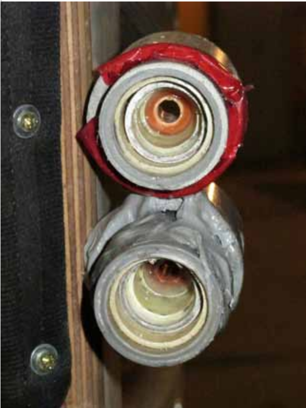
Fig. Trumpet shape connector for water circulation tubes
