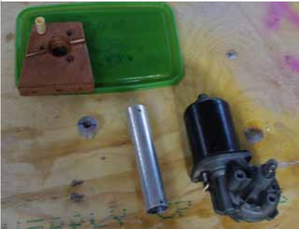
Fig. Motor, shaft, coupling, lid and wooden support.
