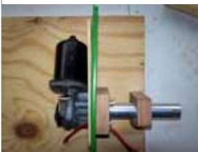
Motor, lid, support and aluminum shaft
