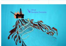
To collect light oil on the surface, repurposed fishing vessels dragged a combination of oil sorbent (white) and oil containment booms (orange). Hundreds of these vessels were deployed by fishermen who exposed their health by manually manipulating the contaminated booms. They would visually spot oil and they would not be able to operate at night, far from shore nor in rough weather conditions.
