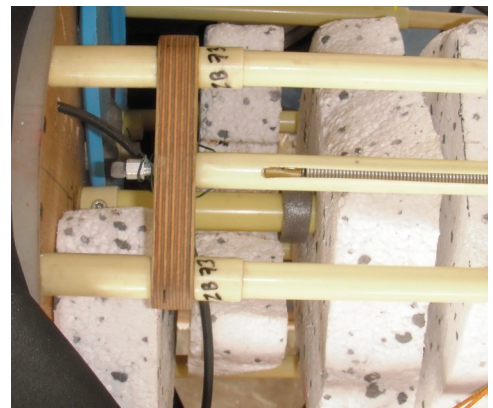
Detail of the top Bowden cable at- tachment to the midships section.
