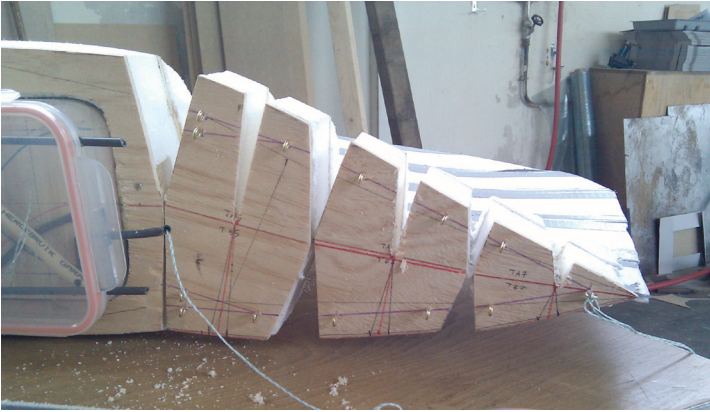
The segmented, articulated bow of Protei_005.3
