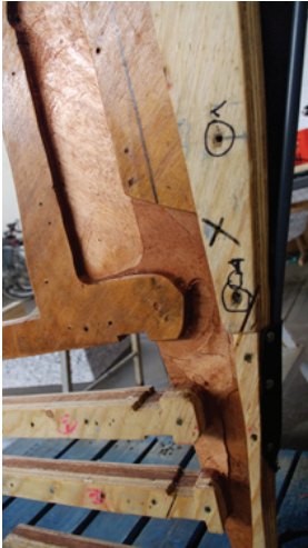
Cut out for the cable routing
