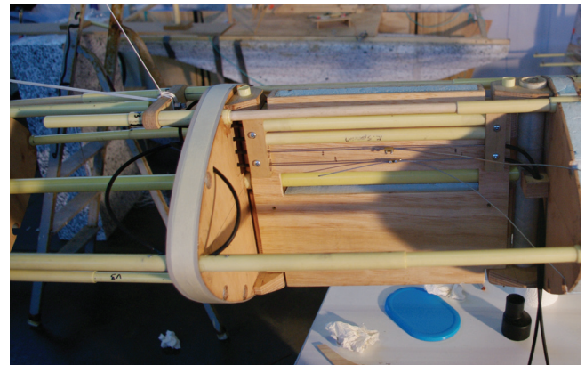
Detail of the midships starboard compartment showing lateral Bowden cable connections.
