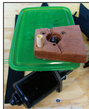
Motor, lid and wooden support assembled
