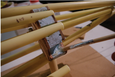
Gluing actuation tubes to bulkheads.
