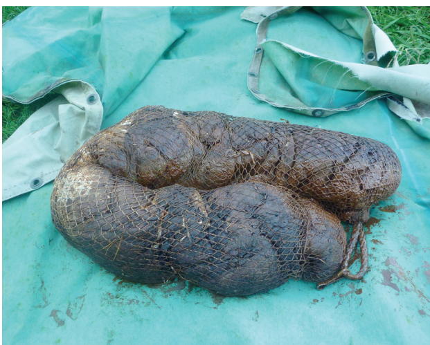
Oil boom saturated with oil
