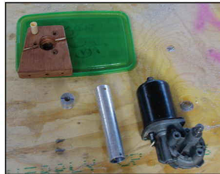
Motor, shaft, coupling, lid and wooden support
