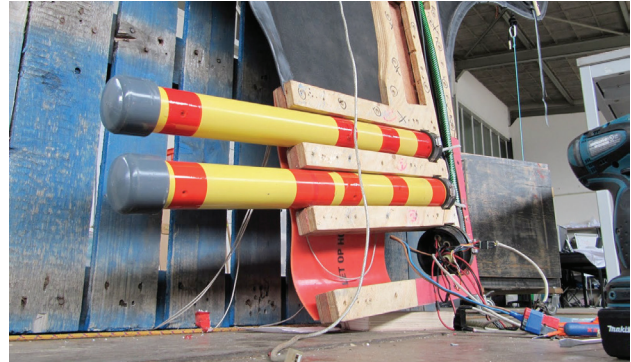
Mounting the linear actuator to the keel
