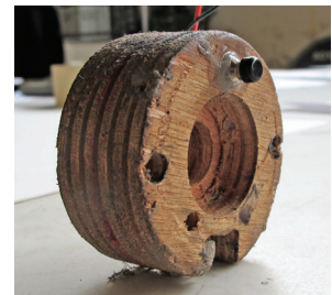
An image of the limit switch used in the old design of the linear actuators.
