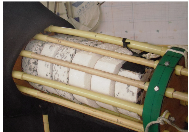
Adding flotation to the hull
