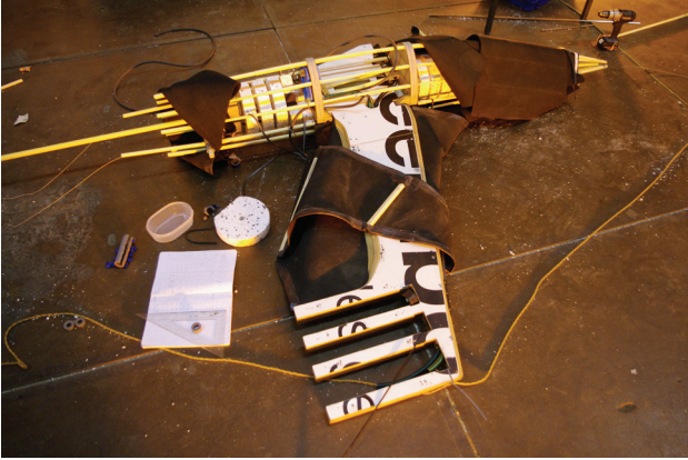
Flexible keel attached to wood keel
