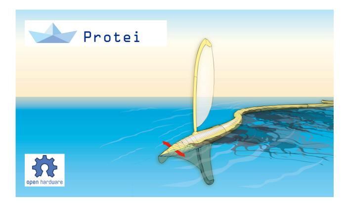
Protei is a Sailing robot that senses and cleans up oceans. Beyond being an autonomous sailing robot, what makes Protei so special is its shape-shifting hull.
