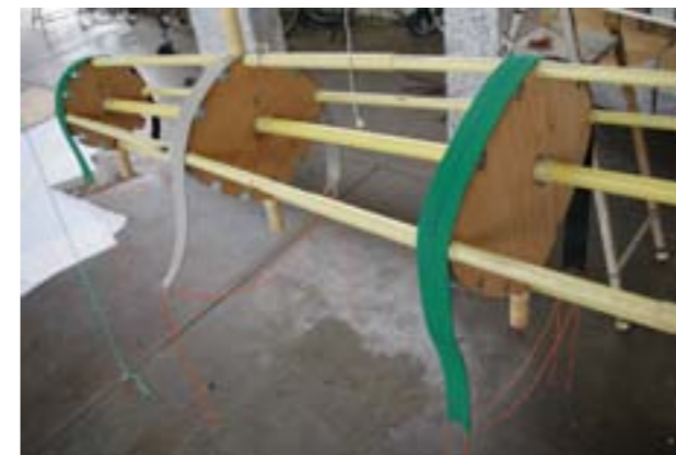
Rubber and textile belts around bulkheads with orange tension lines (left) and rivets (right)
