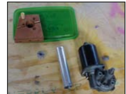
Motor, shaft, coupling, lid and wooden support
