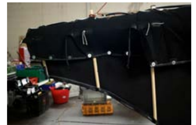
Finishing the skin, by connecting through the keel
