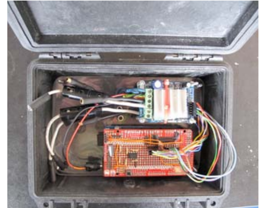
The mounting of the Arduino Mega (with shield), and the two motor drivers (stacked on top of each other) inside the waterproof Pelicase. The colorful cables on the right connect the shield to the motor drivers, and the thick wires on the left provide connections for the motor cables (which enter through a tube on the back of the Pelicase).
