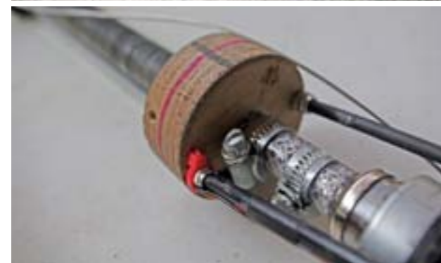
Details of the flexible joint connection between the planetary gearbox and the threaded rod
