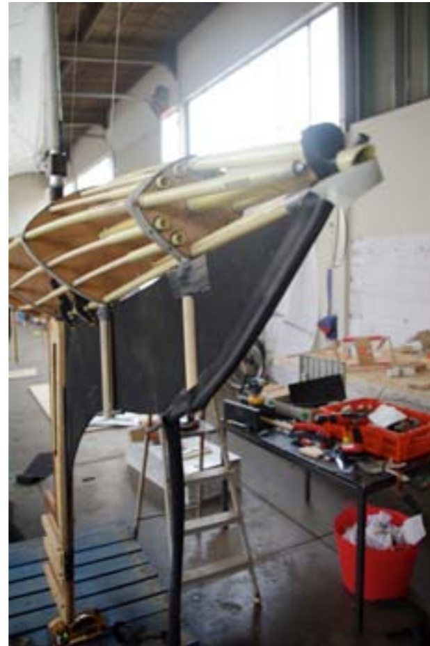
Rubber reinforcement on keel's edge
