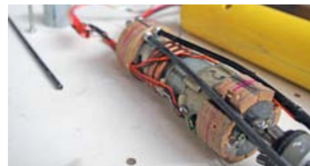
Details of the linear actuator, showing motor mounting, the cooling tube, and cable routing
