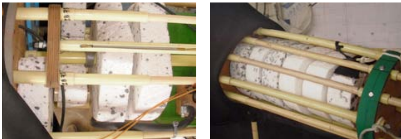
Adding flotation to the hull
