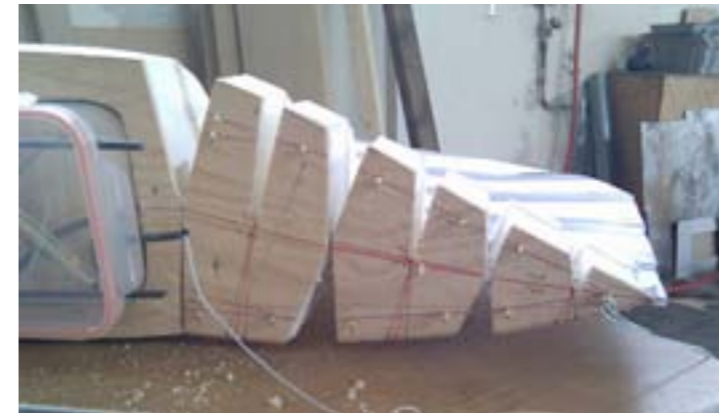
The segmented, articulated bow of Protei_005.3
