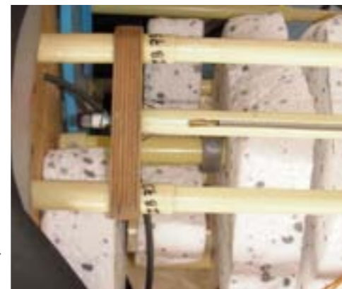
Detail of the top Bowden cable attachment to the midships section.
