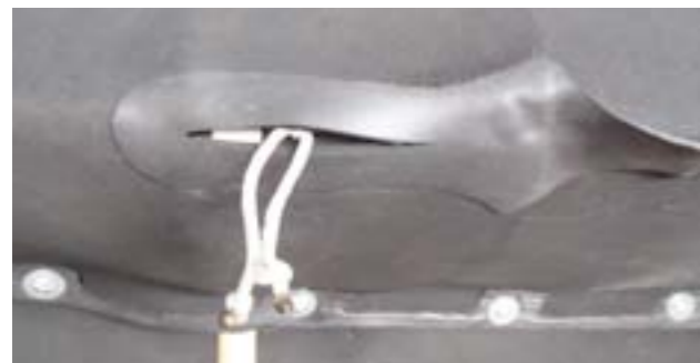
Above: the skin with a connection patch, and the pattern for constructing the patches. Below: slits in the connection patches, and attaching the straps.
