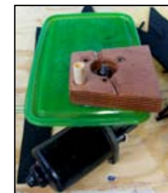
Motor, lid and wooden support assembled
