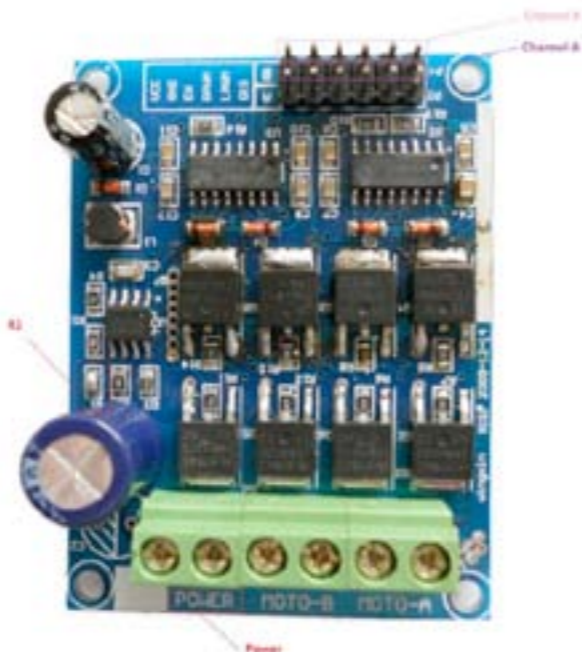
The motor driver board used for driving the actuators on Protei.
