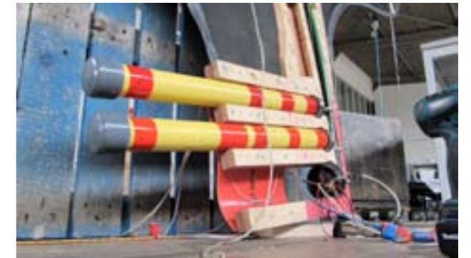
Mounting the linear actuator to the keel
