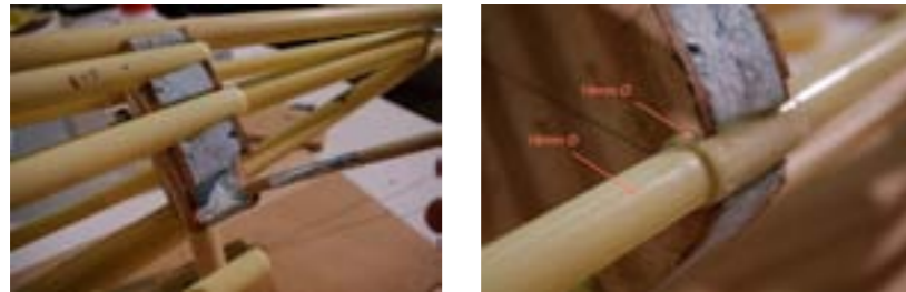
Gluing actuation tubes to bulkheads.
