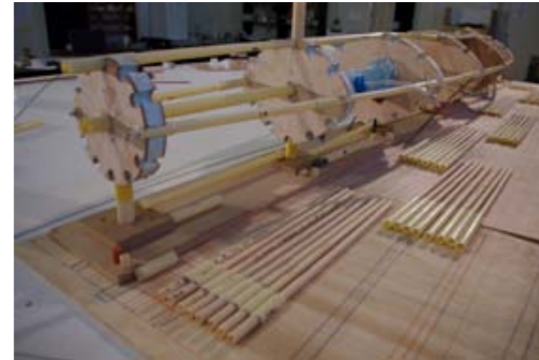
Hull alongside the glued passive spines ready to be inserted.
