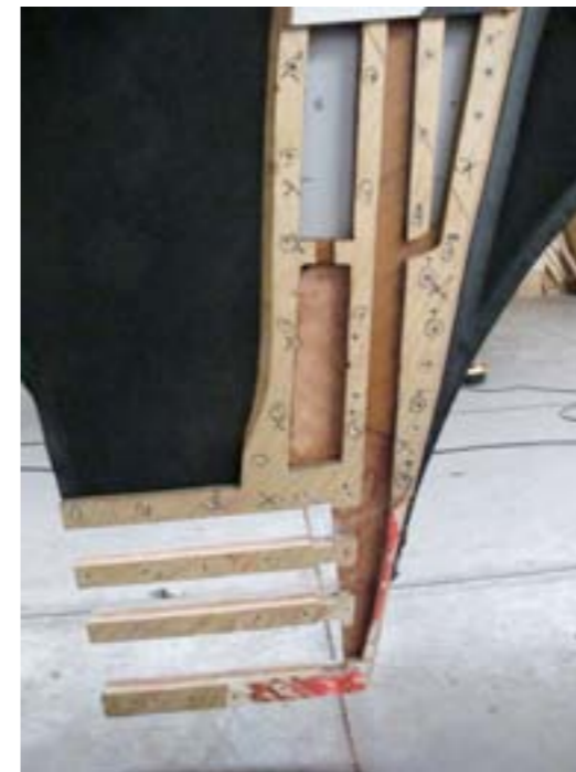
This cutaway view of the keel shows the channel that the hose runs through, inside the keel.
