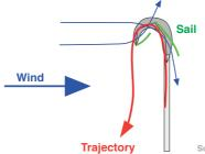
By having a main sail and a jib on a boat that curves means that the relative angle of these sails will change when turning. When tacking the jib catches the wind faster. When jibing the main sail switches side faster. One of the major advantages of a curved hull is that both sails can never be in irons at the same time, which means you have **constant pulling power** from the sail to pull something long and heavy. (oil absorbent boom / scientific payload).
