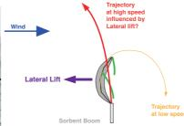
At sufficient speed a curved hull may acquire hydrofoil properties. Instead of vertical lift Protei could produce **lateral lift** meaning the possibility of sailing closer to or further away from the wind therefore more relative motion to the wind and more speed.
