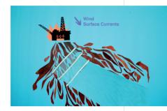
A solution would be to drag successive layers of sorbent dragged upwind, capturing oil drifting downwind. But it is very difficult to move such a large unstable structure against the strong wind and surface currents.
