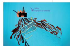
The initial concept for Protei was to pull a long oil sorbent boom behind a sail boat that would tack upwind, capturing the oil drifting downwind in the successive folds of sorbents.
