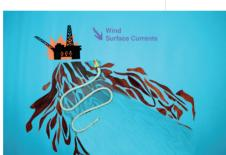
To collect light oil on the surface, repurposed fishing vessels dragged a combination of oil sorbent (white) and oil containment booms (orange). Hundreds of these vessels were deployed by fishermen who exposed their health by manually manipulating the contaminated booms. They would visually spot oil and they would not be able to operate at night, far from shore nor in rough weather conditions.
