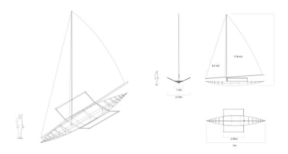
We had several requests for a two-passengers Protei. This is our initial design concept. A 7m dinghy, with a segmented hull equipped with overlapping fish-like flexible scales, generous sail surface area, 2 large trapezes, and a very small closed hull volume, like a <u>windsurf</u> or a <u>moth</u> to easily plane. There would be no rudder tiller but sheets to control the "trim of the hull". The design will continue to evolve over time.
