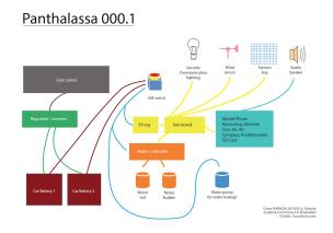
In this early prototype stage, we would use only conventional parts: regular marine-graded solar panels and accessories, car windshield wipers motors on worm gear, Android phone and ioio breakout board, windsurf mast on bearings, fiberglass hull construction... If we make this machine longer -4m for instance- it could be a truly competitive blue water vehicle for ocean science (see "Competition" p.17).
